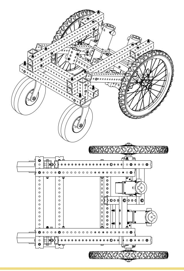
4 Install the shocks using the shock brackets on the frame. Install the chair platform.
