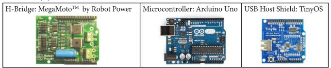
In our prototype we used an Arduino microcontroller in combinations with a MegaMoto<sup>TM</sup> H-bridge. To incorporate USB devices such as a joystick, we also used a USB host shield. These three boards are designed to stack on top of one another. The configuration of these boards is shown in the block diagram.
